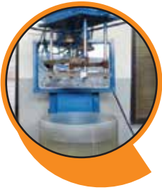
Porosity Test Bench for G-4 Meter Parts
