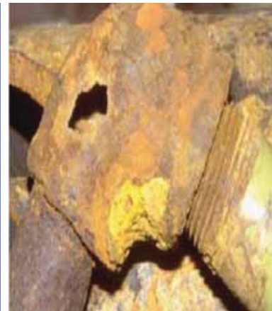
Above ground corrosion leak
