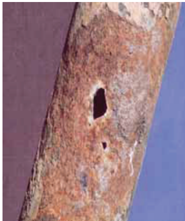
Underground corrosion leak
