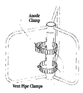
Figure 1: CENTRALIZER FRAME (MS WITH WELDED CLAMPS FOR ANODE AND PVC SLOTTED PIPE)
