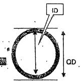
Washer shall be made from Neoprene material. Only fresh material shall be used, recycled material will not be acceptable.
