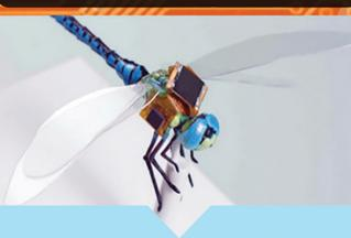
Engineers have fitted dragonflies with tiny, backpack-mounted controllers that issue commands directly to the neurons controlling the insects' flight. Backpack system includes energy harvesting, navigation and optical stimulation.
