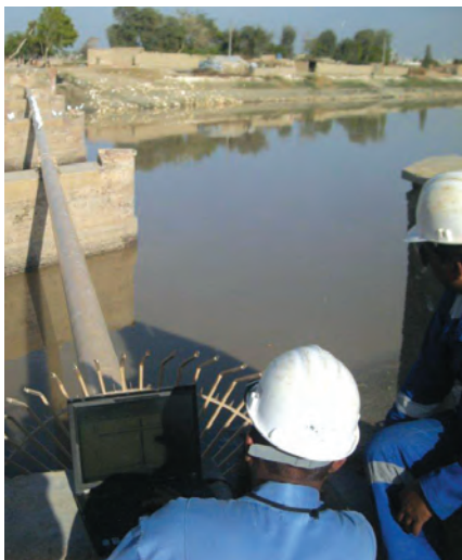
LRUT on 16" dia on Dadu Canal overhead
