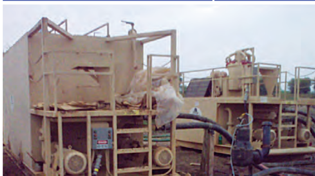
Mud Mixing and Recycling Units
