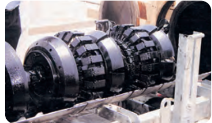
Intelligent Pigging carried out between Nawabshah HQ2 to Karachi Terminal in fine segments by SSGC and Rosen Inc. engineers.
